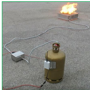
GF42 and its solenoid valve module using the wireless remote control option
