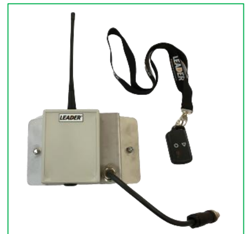
Aeros 2 using the wireless remote control option
