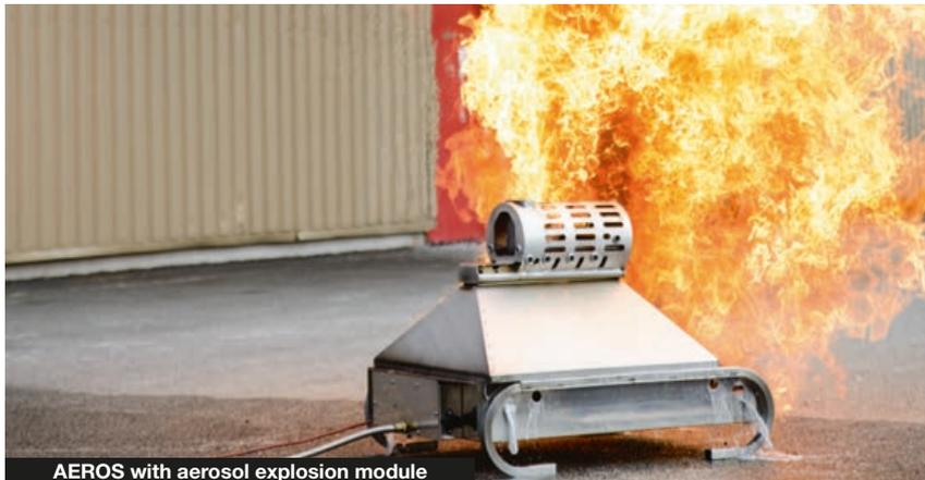
**AEROS with aerosol explosion module**
